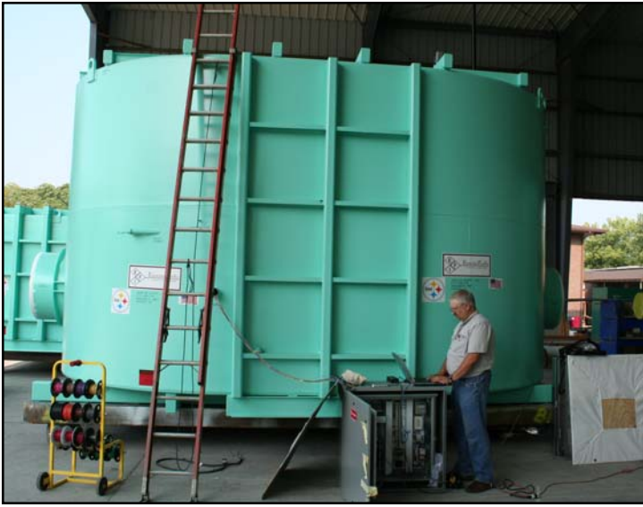
This picture shows Mike Johnson, one of EFI's Control System Designers/Programmers exercising the control system and the valve solenoids as part of the final QA checkout.
