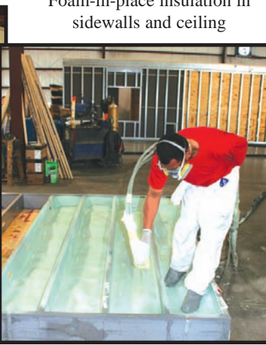
Jig built, ASTM steel framing for walls & ceiling with interior plywood sheathing
